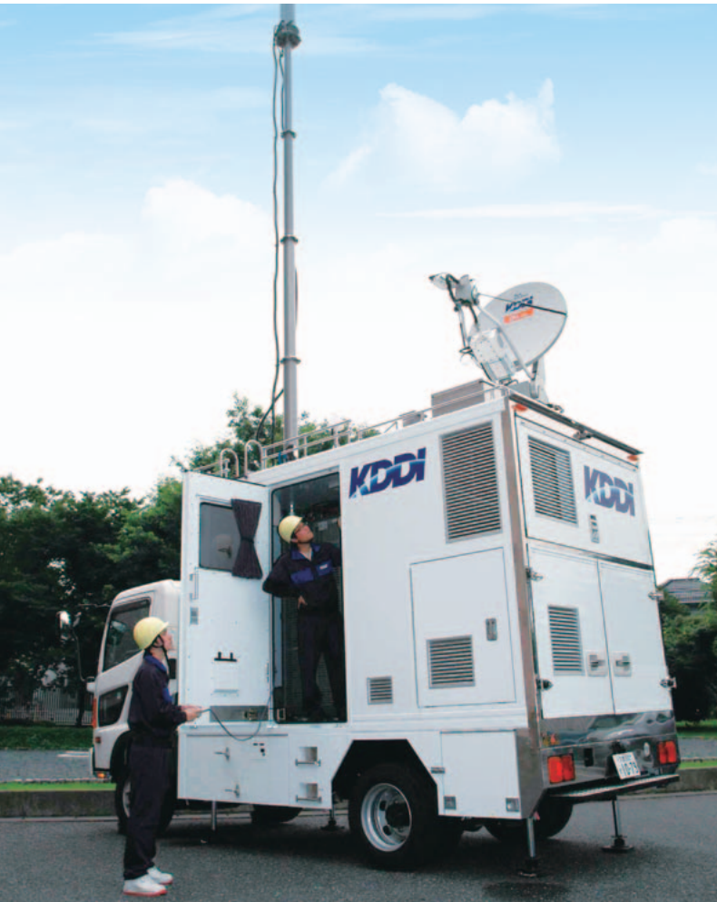
Vehicle – mounted satellite base stations – these are a powerful tool for keeping the communications network up in times of disaster or other emergencies.
