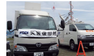
Mobile power supply vehicles and vehicle-mounted satellite base stations provide a communications infrastructure in disaster-stricken areas
