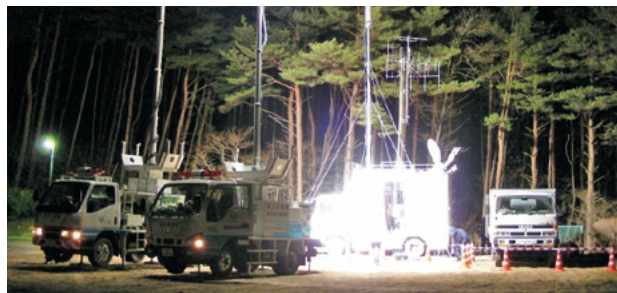
Vehicle base stations (Rikuzentakata, Iwate Prefecture)
