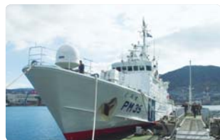
Satellite antenna (inside the cylindrical cover) toward the bow of the patrol vessel Kurose Source: Study Team for Shipboard Installation of Mobile Phone Base Stations for Use in Emergencies
