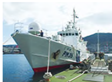
Satellite antenna (inside the cylindrical cover) toward the bow of the patrol vessel Kurose Source: Study Team for Shipboard Installation of Mobile Phone Base Stations for Use in Emergencies
