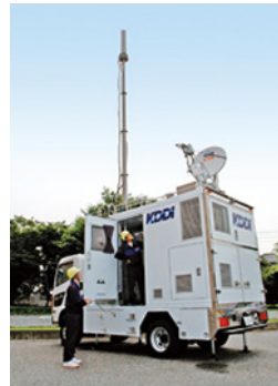
Vehicle-mounted base station
