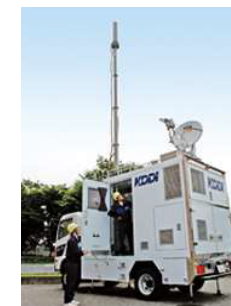
Vehicle-mounted base station
