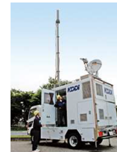
Vehicle-mounted base station
