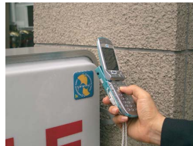
Testing the utility of RFID tags
