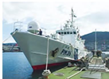
Satellite antenna (inside the cylindrical cover) toward the bow of the patrol vessel Kurose
