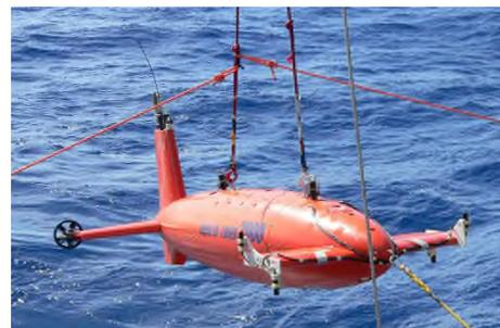
AE2000 underwater robot equipped with hydrophone array on wings
