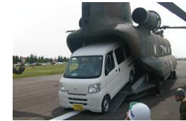
Self-Defense Forces use a large helicopter to transport a mobile base station in an exercise conducted in Tohoku.
