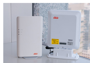
au Femtocell (left) and au repeater (right)
