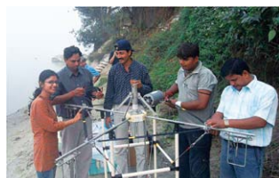
Assembling a hydrophone (underwater microphone) array
