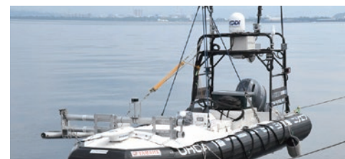
▲An unmanned boat. This robotic vessel transmitted the data received from the autonomous underwater robots in the ocean via satellite communication. It proved that remote operation via satellite communication is possible.
