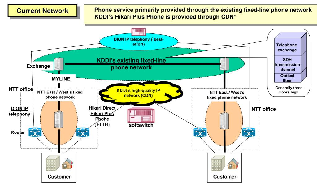
\*CDN (Contents Delivery Network) integrates data and voice, prioritizing the transmission of voice over data so that the quality of the telephone calls are equivalent to that of existing fixed lines.
